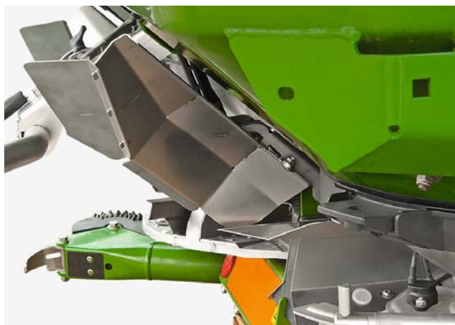
Border spread deflector folded upwards
