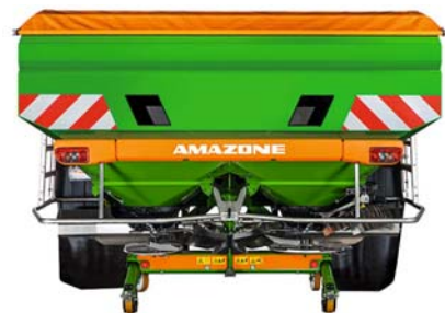
L 4200 extension (filling width 2.71 m) with foldable ladders
