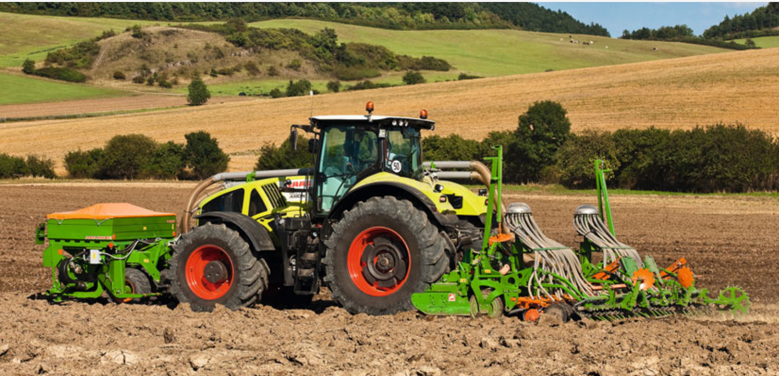
Avant front tank drill combination; 6 m working width
