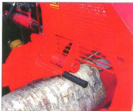
The spring-loaded support roller automatically opens the guard.
