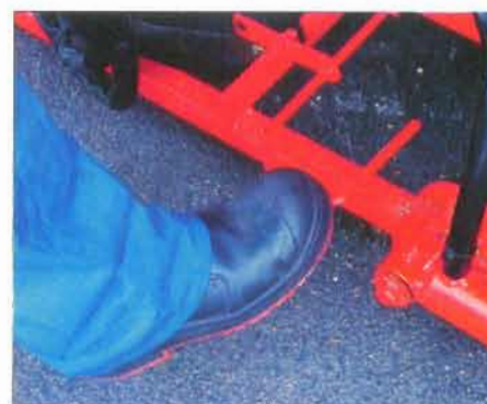
Triggering the splitting movement by foot.
