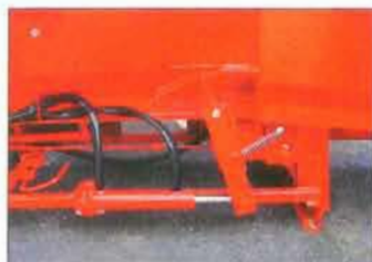
Hydraulically adjustable splitting blade.
