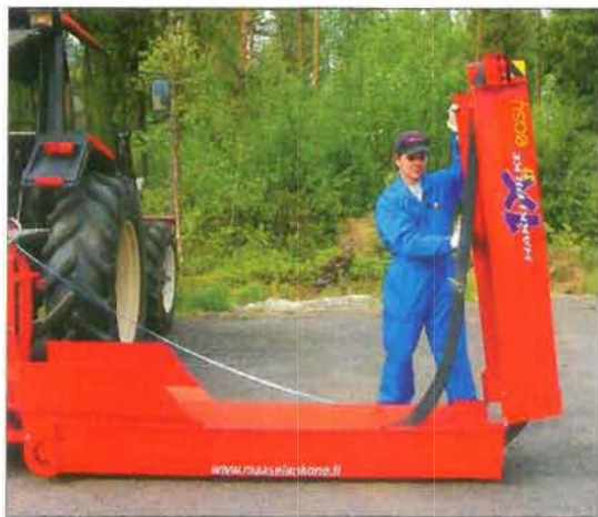
The 4 m conveyor folds easily for transport.
