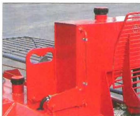
Automatic oiling of the cutting chain. Oil goes to the chain only when the machine is in use. There are separate tanks for the chain oil and hydraulic oil.
